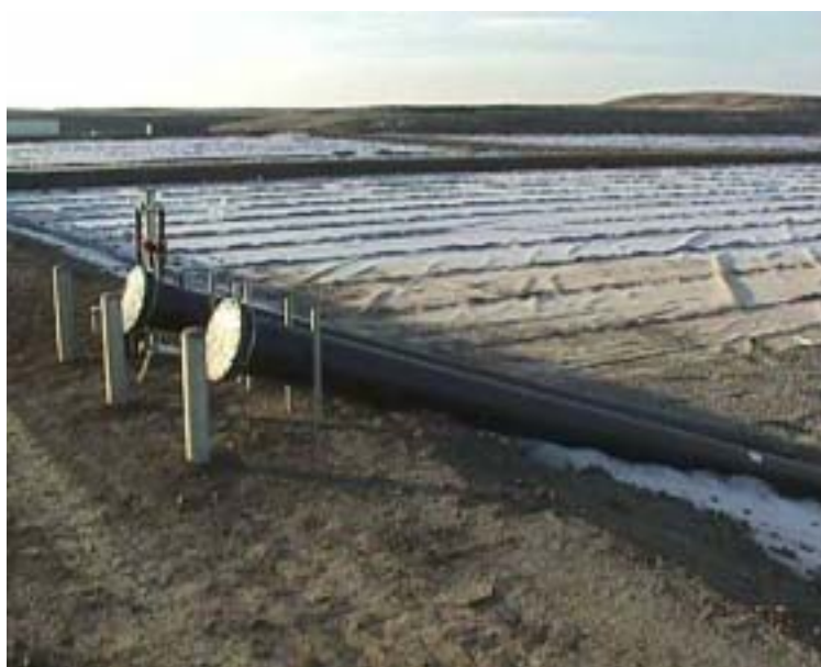
Yolo County landfill is the test site for a new method of anaerobic decomposition to accelerate the production of methane for fuel. This project is funded by SMUD's ReGen program.
